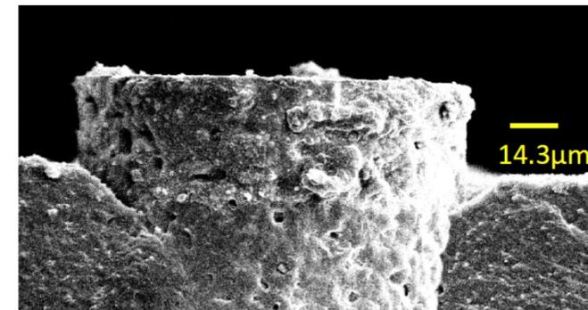
Glass-based filler was dissolved by HF, leaving pores in Au
