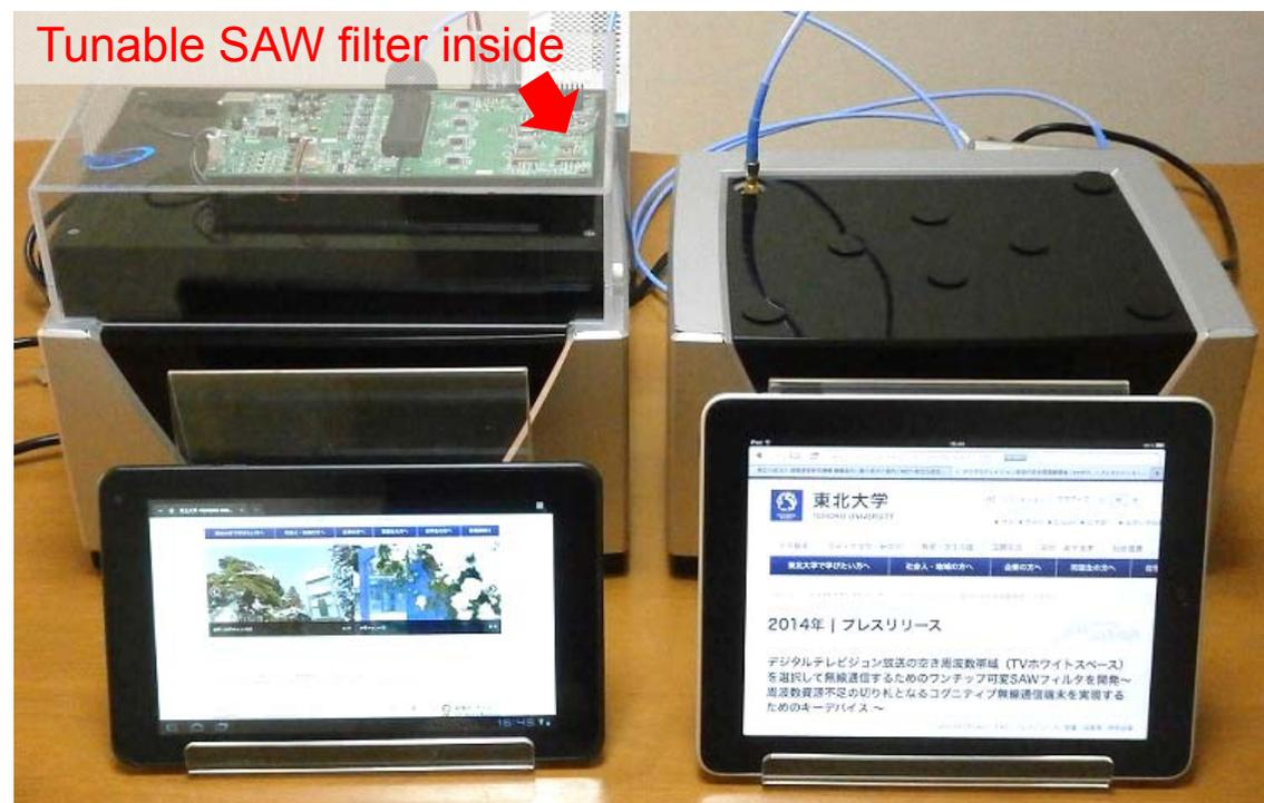
Tablet PC for interface connected to the terminal cognitive wireless system
