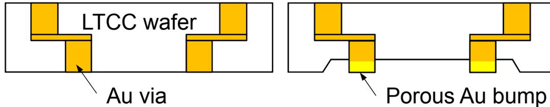
1) Production of LTCC wafer 2) Wet etching of LTCC wafer to make cavities
