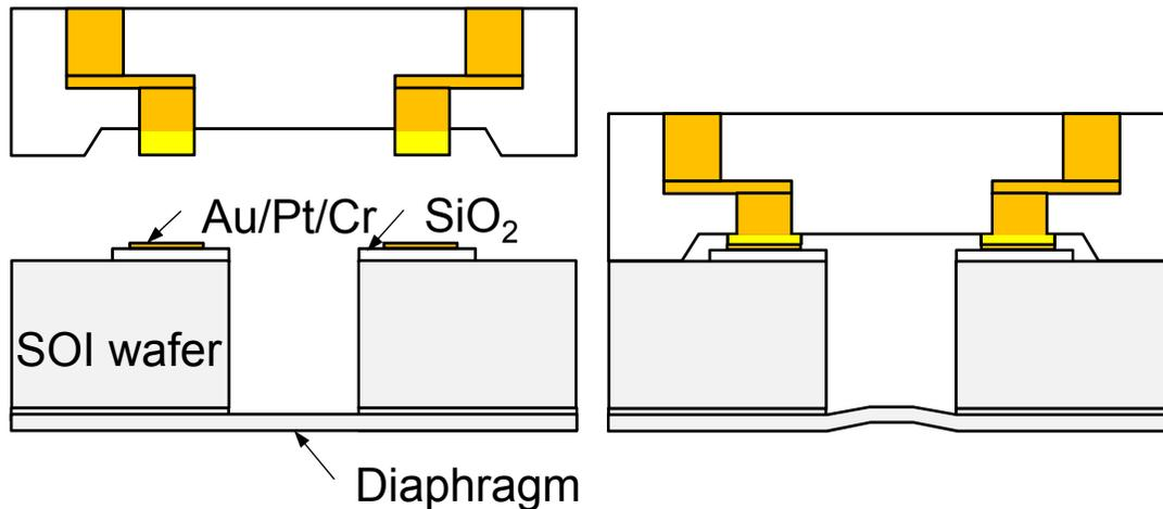
3) Wafer alignment 4) Anodic bonding with electrical connection
