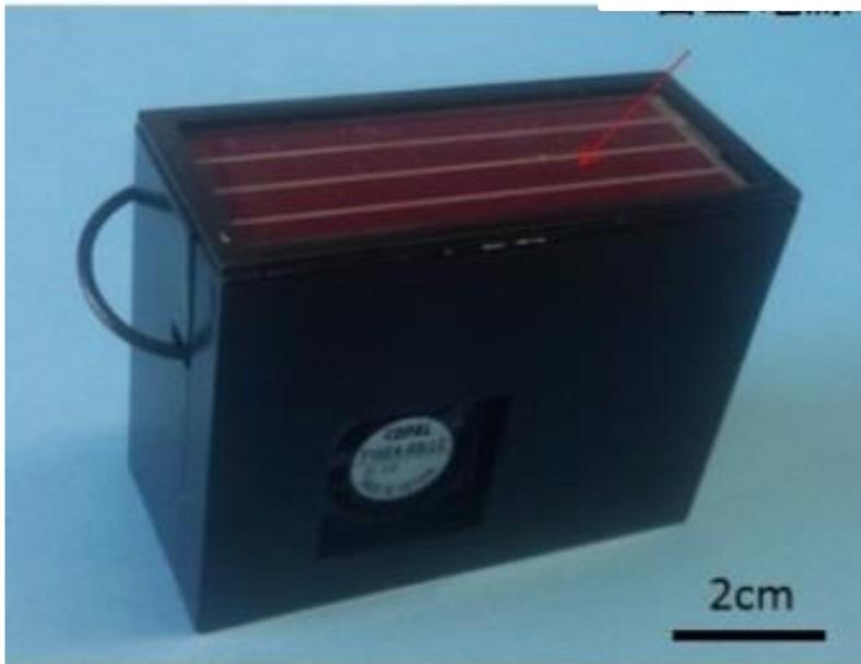
▪ Development of Particle sensor triggered by event driven Piezo-electric switch (average PC =  $95 \mu W$ )
