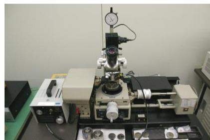
Spreading resistance measurement
