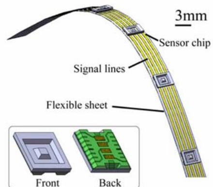
Tactile sensor chip and signal line
