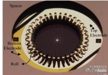
(b) Single actuator with the spacer
